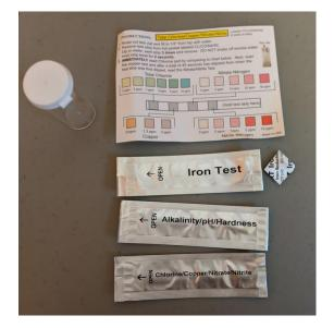
**Figure 2.** Contents of the lab kit sent to each student to test water quality at home. Included were instructions, sample vial, test strips, and iron tablet, all provided by Test Assured [4].
