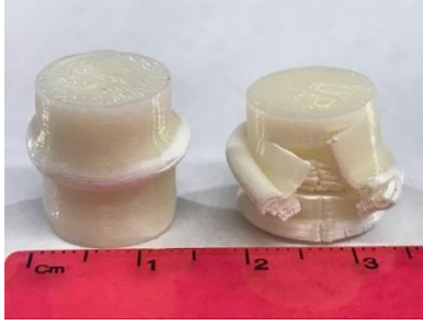
Figure 22. ABS Specimens of Sparse Structure Printed by Mojo at Upright Orientation After Compression Test.
