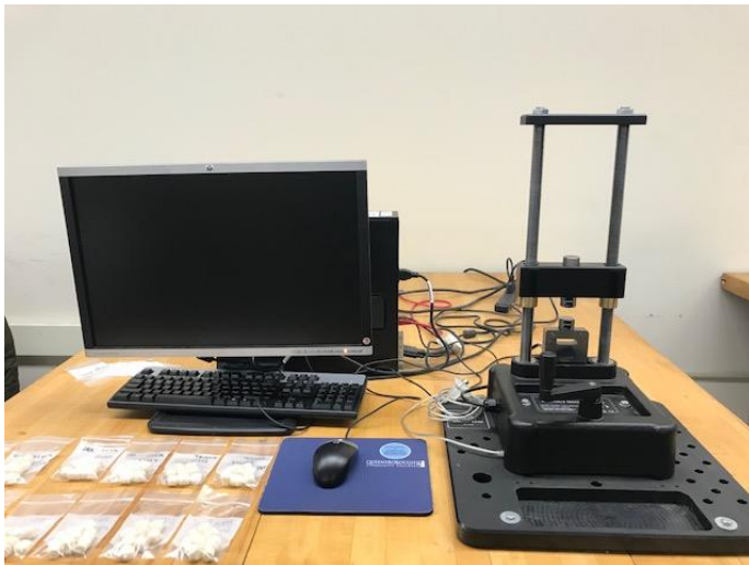
Figure 6. PASCO ME-8244 Comprehensive Materials Testing System
