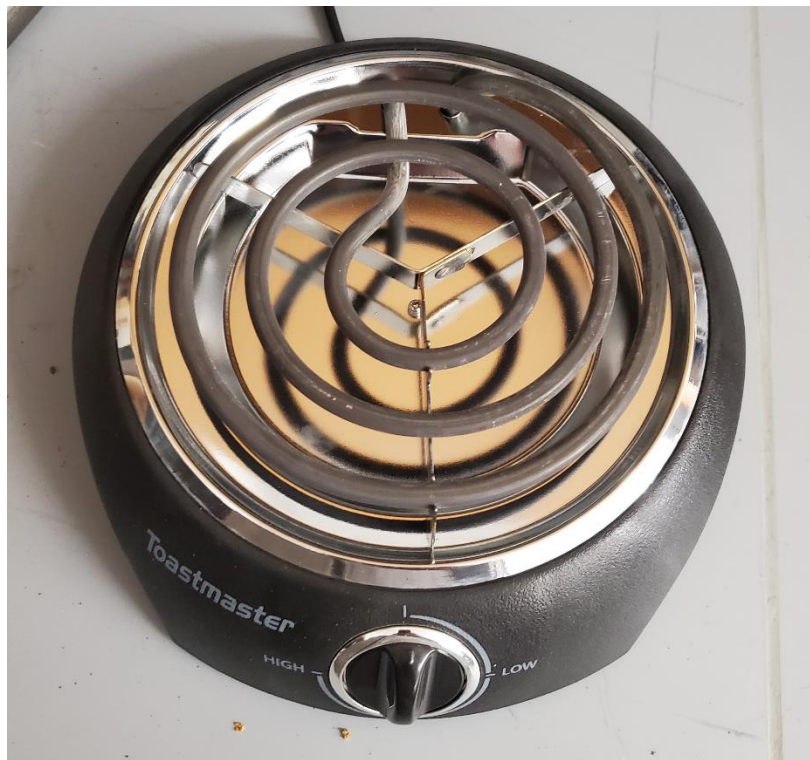
Figure 2 shows the hot plate used for the heat source
