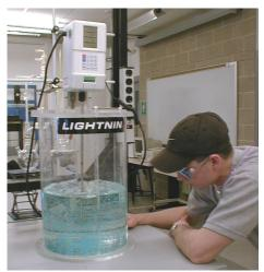
fabricated in-house. This makes a great experiment for a fluid mechanics/transport class or process component design course.
