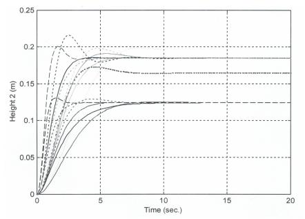
Figure 7: Simulation of plant with state-feedback for nominal and extreme cases.
