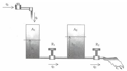
Figure 1: A two-tank liquid-level system.
