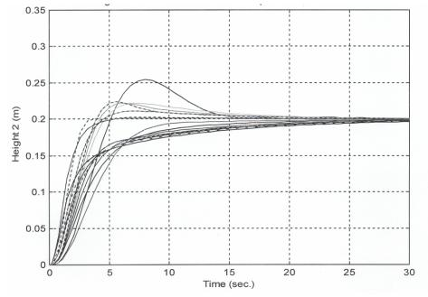
Figure 5: Closed-loop system response with PID controller for 16 extreme cases
