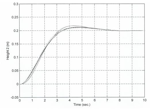
Figure 9: Responses of plant and state feedback with integral control for nominal and extreme cases.
