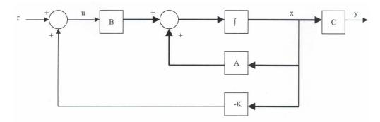
Figure 6: Plant with State Feedback
