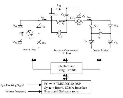
Figure 1. Circuit schematic of the single-phase system
