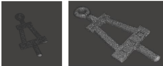
Figure 17. Mesh reduction in Meshmixer
