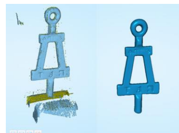
(A) (B) Figure 16. Point cloud to STL conversion
