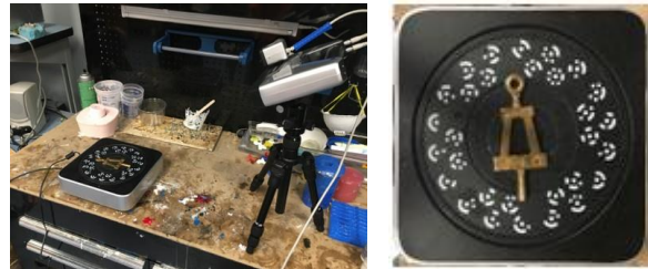
Figure 14. Orienting part on rotary platform
