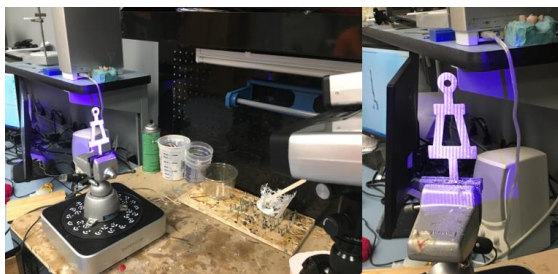
Figure 15. Alternative orientation of powder-coated part in fixture
