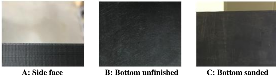
Figure 22. Surface finish of FDM model and post-processing
