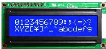
FIGURE 4 16X2 LIQUID CRYSTAL DISPLAY MODULE.
