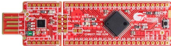
FIGURE 3 PSOC 4 CIRCUIT BOARD (“PROTOTYPING KIT”).
