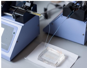
Figure 1. A typical microfluidic chip connected to two syringe pumps.
