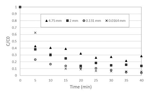
Figure 2. Changes to turbidity concentration, normalized to initial NTU, over time for varying sized granular media. Smaller grain-sizes correlated with faster turbidity removal and lower stabilized effluent turbidity, though head loss was severe.
