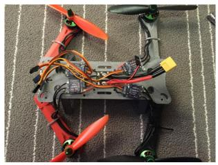
Figure 14: Motors Attached to the Arms
