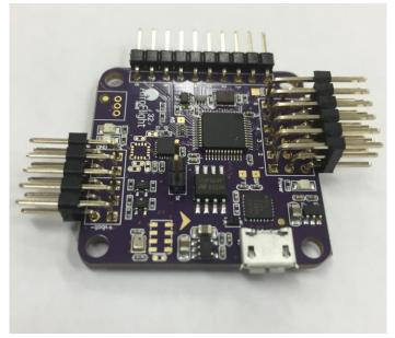
Figure 11: Completed Flight Controller
