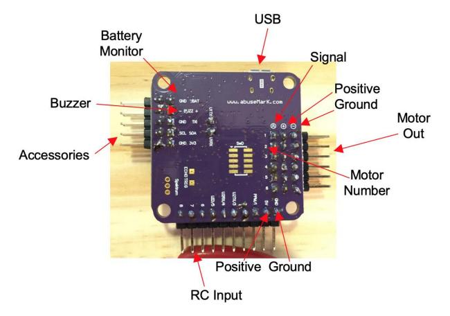
Figure 12: Flight Controller Setup
