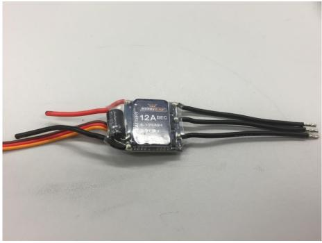
Figure 3: Electronic Speed Controller (ESC)
