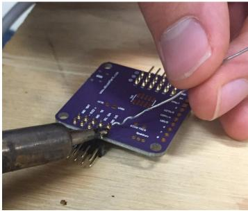
Figure 10: Solder the Pins to the Flight Controller
