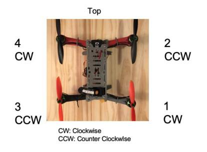
Figure 13: Motor Numbers and Directions
