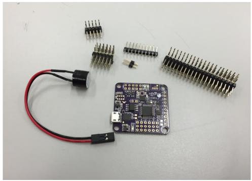
Figure 2: Flight Controller and Piezo Buzzer
