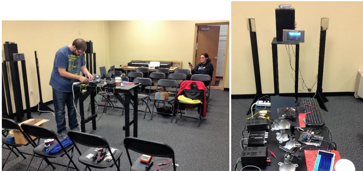
Figure 5. Preparation for the Laser-Music “Concert” continued. Left photo with Engineering Team members Rokosky and Rickman (L to R) making final product and performance-room arrangements. Right photo featuring the Laser-Music product laser and electronics (on table) and 5ft moveable wooden stands with optical detector with audio amplifier and speaker (center) and angled mirrors (left and right of center) directed at optical detectors with audio amplifier and speakers located to the left and right outside of the image.
