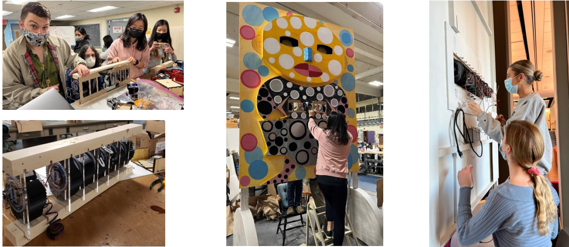
Figure 2: Construction of the 8-character split-flap display: (left top and bottom) as a standalone structure, (center) preparing for insertion in Think Bot, and (right) completing the final electrical wiring.
