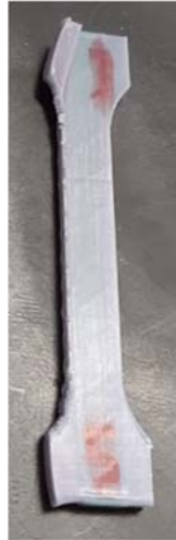
Figure 6. Chipped Test Specimen
