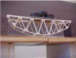
Figure 3: Bowstring Deck Truss made of Manila File Folder<sup>13</sup>
