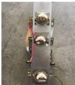
Aluminum arm with the nozzles install
