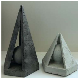
Figure 11. Casting produced by gray iron lost foam (left) and aluminum investment
