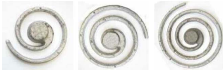
Figure 10. Casting produced by aluminum 356 at different temperatures using gravity casting
