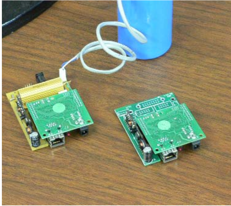
Figure 3. Two embedded Ethernet controllers with Power-Over-Ethernet (POE) capability, for reporting power statistics for the roof-top PV and turbine.
