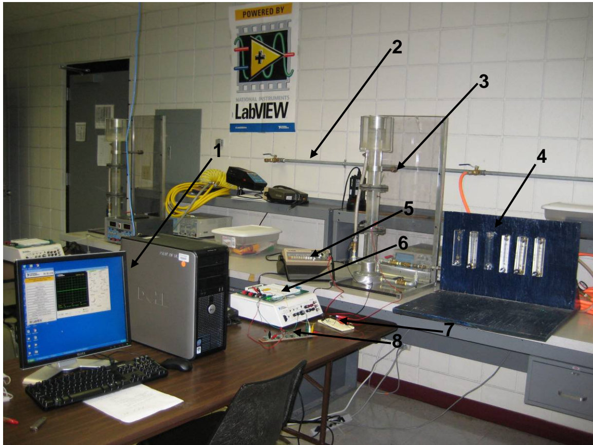
Figure 4. Experimental System Consisting of 1) Computer-Aided Data Acquisition System, 2) Compressed Air Line, 3) Vertical Column, 4) Rotameters, 5) Function Generator, 6) NI ELVIS with Prototype Board, 7) Wheatstone Bridge, and 8) Professional Low-Pass Filter
