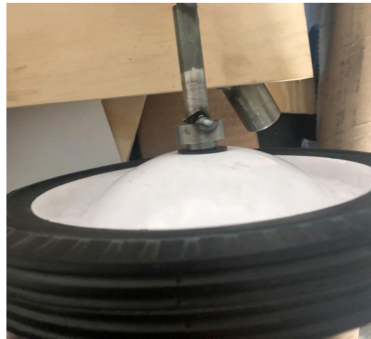
Figure 5: Metal stopper attached to trucks
