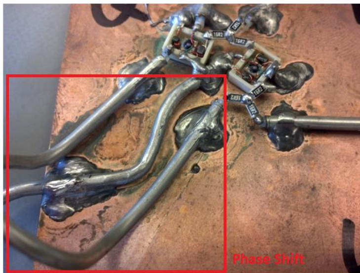
Figure 4: This photograph shows additional detail on the 90 degree phase shift section of the I-Q modulator. The local oscillator input comes in on the right hand side of the photograph. The Y-network power splitter then puts one output signal directly on the “I” mixer. The red box in the photograph highlights the additional coaxial cable section length that is used before the local oscillator is applied to the “Q” mixer.
