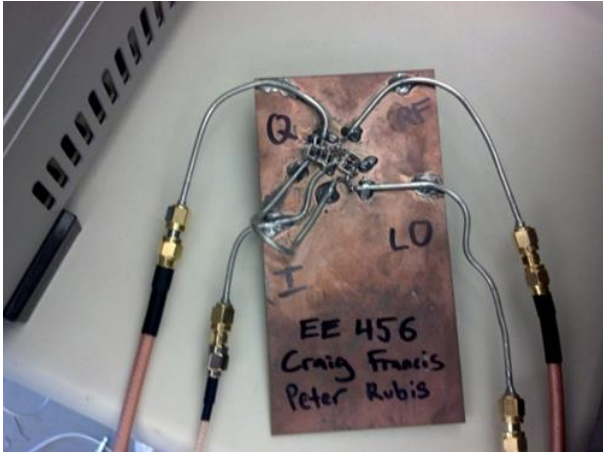
Figure 2: This is a photograph of a completed I-Q modulator assembly. 0.085 inch semirigid coaxial cable assemblies are soldered on to a printed circuit board ground plane. The surface mount mixers are mounted upside down (dead bug construction) and interconnect to the coax and to the power splitters. The power splitters are made from three 16 ohm surface mount resistors in a Y network but are hard to see in this photograph. Figures 3 and 4 show the detail of the soldering around the mixers much better. The 4 ports of the I-Q modulator are labeled. The "LO" or Local Oscillator port controls the switching of the mixers. The "I" and "Q" ports are used as data inputs or data outputs. The "RF" or Radio Frequency port can be used as the modulator output or demodulator input.
