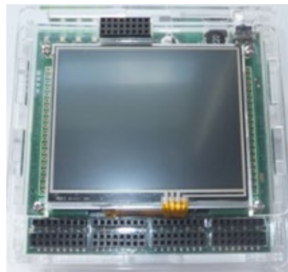
Figure 2: The Proteus microcontroller, which features a touchscreen LCD.
