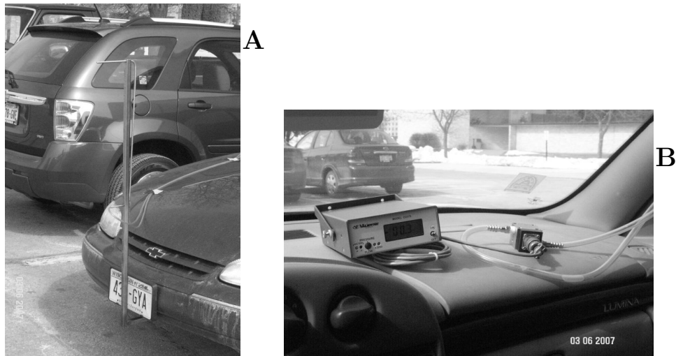
Figure 4: Pitot tube experimental apparatus A) Pitot tube mounted on front of car B) Pressure transducer for reading the dynamic pressure
