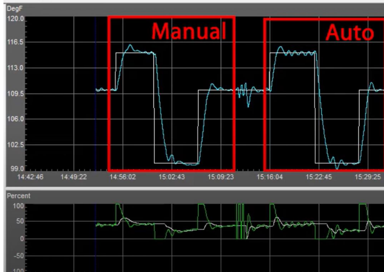
Figure 5 – PID Manual vs. Auto Tuning
