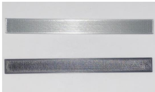
Figure 1: samples with 0-degree (top) and 90-degree (bottom) printing orientations
