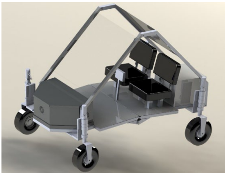
Figure 1: Artist rendering of the designed LTV. This LTV can transport two astronauts and folds at the midsection.
