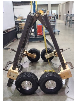
Figure 2: The LTV in the folded position. The four hub motors are used to fold the LTV reducing needed hardware.
