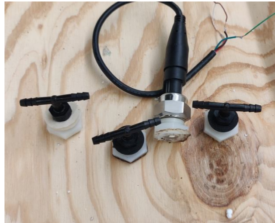
Figure 2: Pressure Sensor and Tank Outlet Ports
