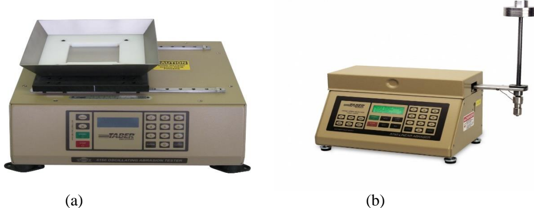
Figure 1. Testing Equipment: (a) Oscillating abrasion tester - Model 6160 [11] and (b) Reciprocating linear abrasion tester – Model 5900 [12]
