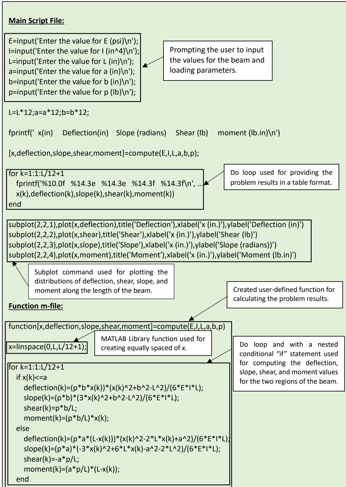
Fig. 3 MATLAB Script File for Analyzing the Beam
