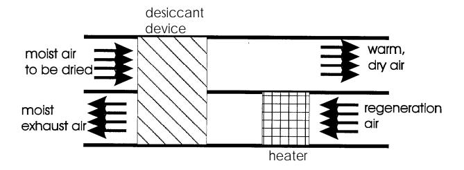
Figure 3. Illustration of the basic components of a desiccant dehumidification system from section B.
