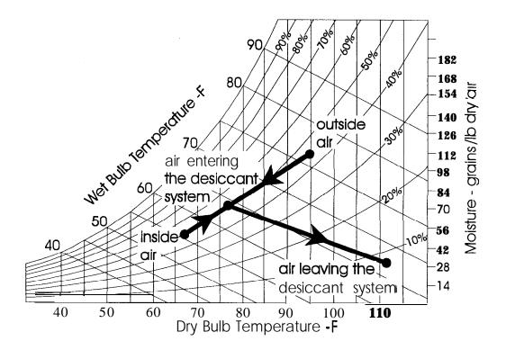
Figure 6. Psychrometric chart showing conditions of the process air in the desiccant system installed in a commissary from section G.
