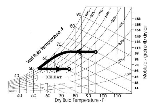
Figure 2. Illustration of the cold-coil dehumidification process on a psychrometric chart from section B.
