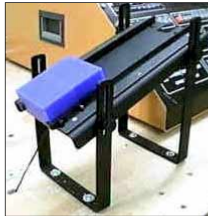
Raw Material Feed Station
