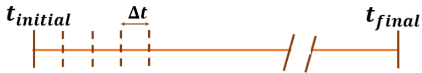
Figure 2: The axis of independent variable is discretized in steps of \Delta t .
