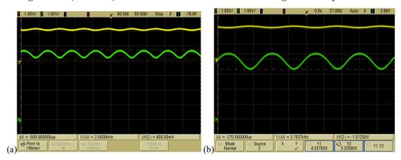
Fig. 7 Common source amplifier working in saturation region with, (a)  $1K\Omega$  load resistor using switch S1 and, (b)  $2.2K\Omega$  load resistor using switch S2. The yellow waveform is small signal input whereas green waveform is the amplifier output.
