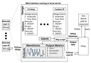
Fig. 1 Overview of our approach. The student will select the design for experimentation (or write a netlist) and enter the options. After submitting the request, a php script will compile the user selections to FPGA bitstream which in turn will apply the settings on the board using available resources. The sampled output from test board is collected by the FPGA and sent back. Multiple students will be able to execute experiments on the board simultaneously to run their test cases independently.
