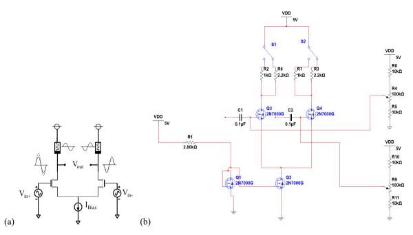
Fig. 6 Schematic of, (a) differential amplifier; (b) proposed reconfigurable differential amplifier with tunable loads and current biasing. The small signal input is applied through capacitor C1 and C2. The analog switches (S1 and S2) are also shown that the students will configure remotely.
