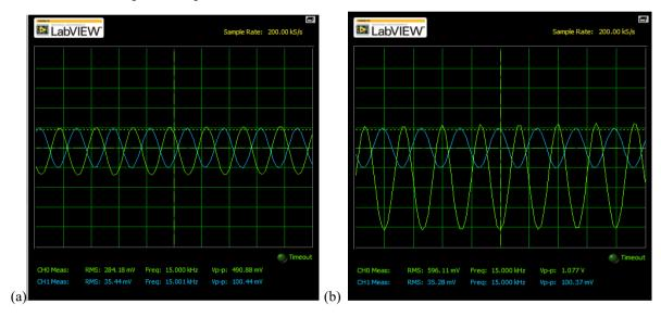
Fig. 9 Differential amplifier working in saturation region with, (a)  $1K\Omega$  load resistor using switch S1 and, (b)  $2.2K\Omega$  load resistor using switch S2. Blue is the input and green is the output waveform.
