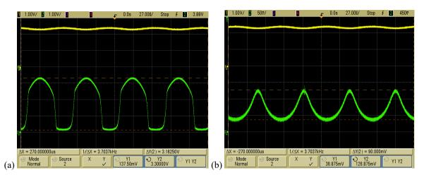
Fig. 8 Common source amplifier working in linear region with, (a)  $1K\Omega$  load resistor using switch S1 and, (b)  $2.2K\Omega$  load resistor using switch S2. The yellow waveform is small signal input whereas green waveform is the amplifier output.
