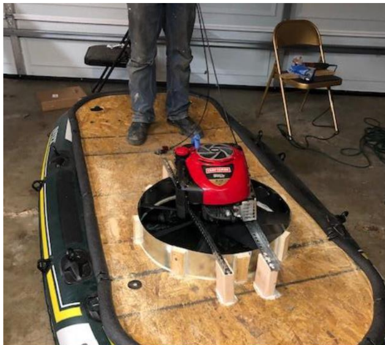
Figure 5 – Physical Assembly of Personal Hovercraft Frame [14]
