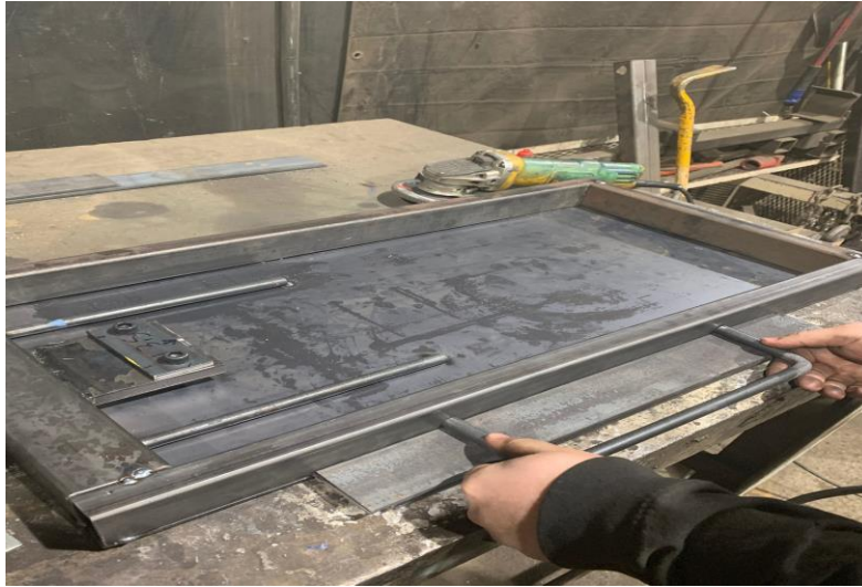
Figure 2 - Physical Build of the Portable Tensile Testing Apparatus [12]
