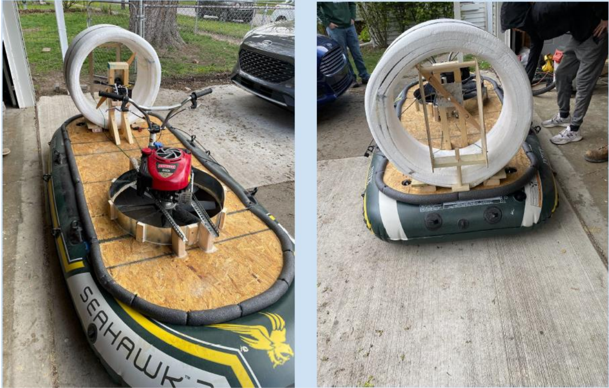
Figure 6 – Full Physical Assembly of Personal Hovercraft [14]
