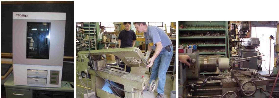
Figure 4. Some processes used in the capstone project: FDM Rapid prototyping machine (left), Cutting (middle), and Machining (right).
