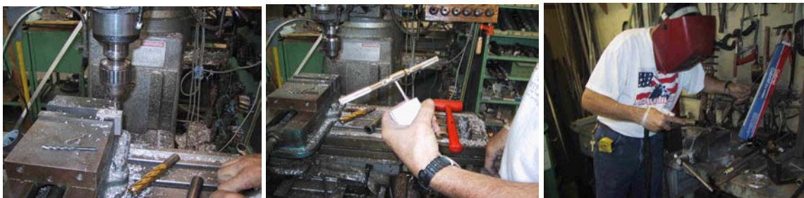
Figure 5. More processes used in the capstone project: Drilling (left), Tapping (middle), and Welding (right).
