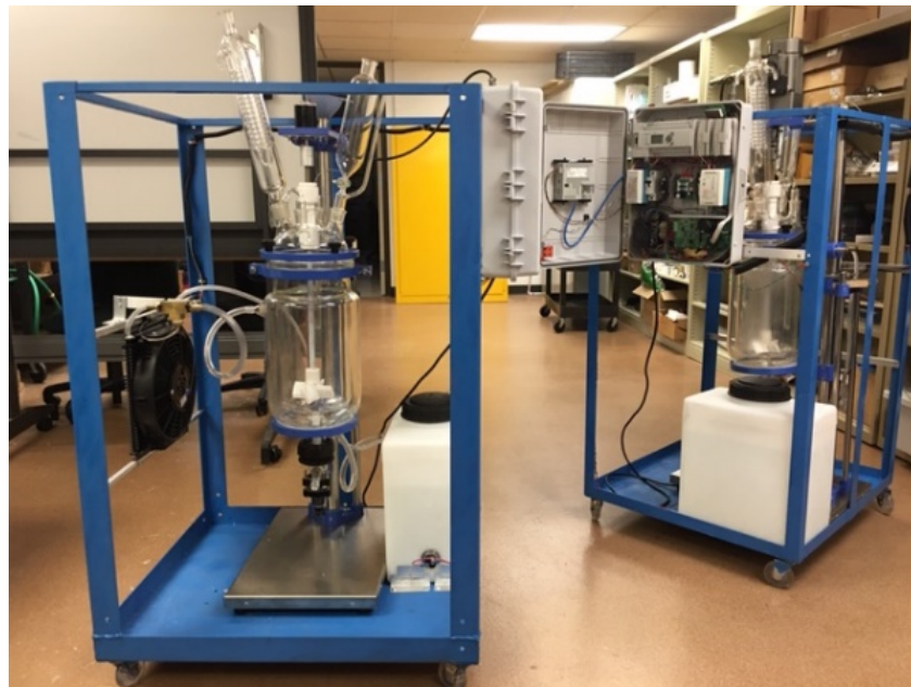
Figure 3: Bioreactors 2 and 3 with PLC based automation
