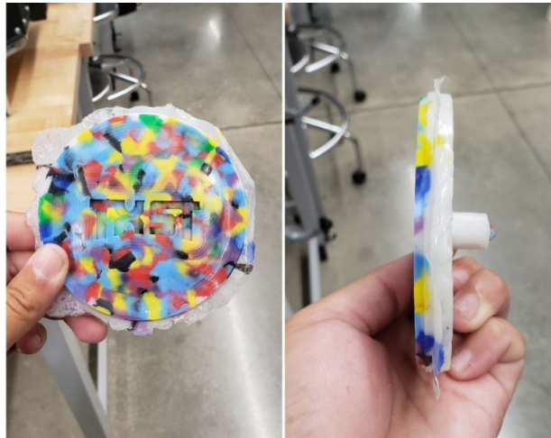
Figure 12: Product after removal from mold
