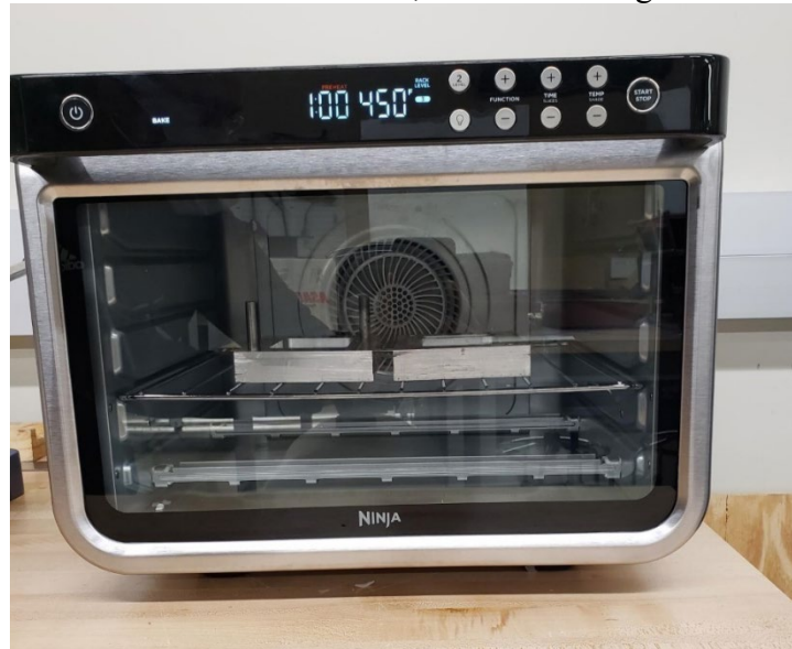
Figure 7: Pre-heating molds (450 °F)
