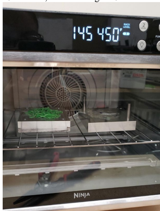
Figure 8: Shredded HDPE melting in mold
