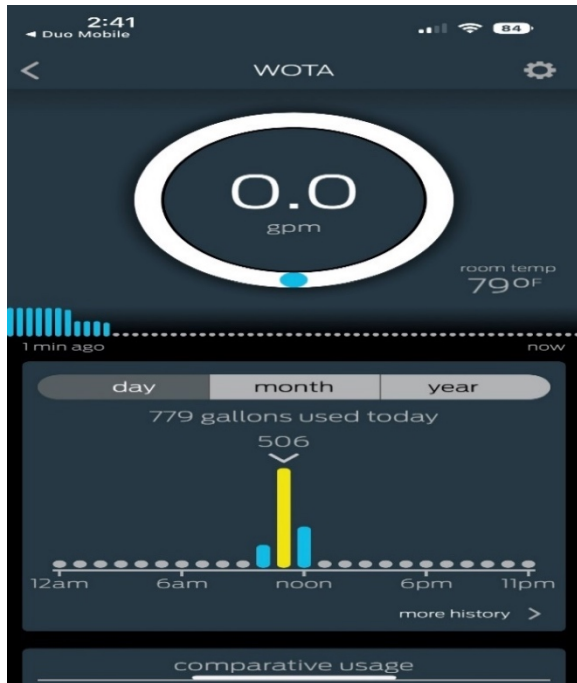
Figure 14: Stramlabs Cooling-Water Flow-Rate Display.
