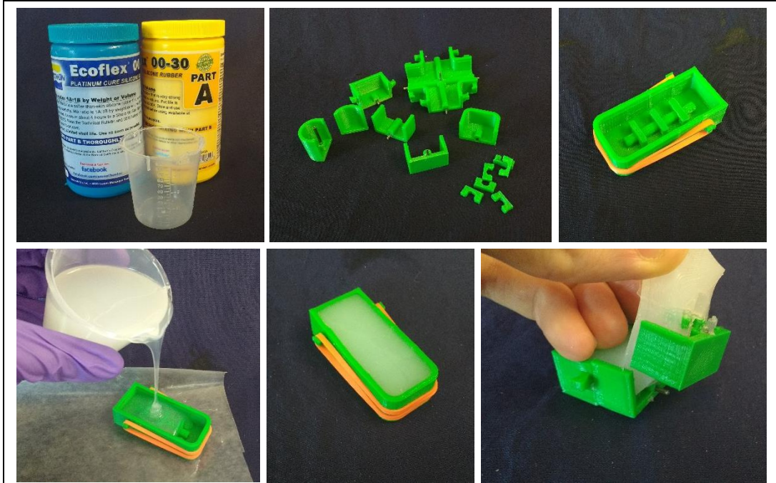
Figure 2. Fabrication phase 1 (from left to right, top to bottom): Ecoflex silicone containers and mixing cup, mold parts, assembled finger design, pouring mixed Ecoflex into the mold, cured finger, and demolding the finger.
