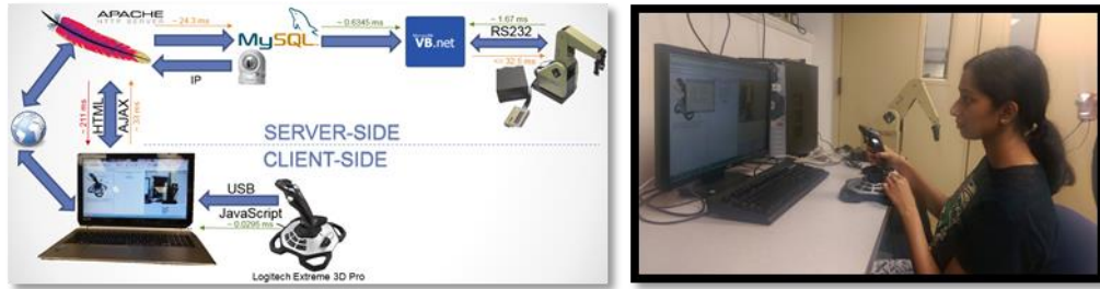
Figure 9. Architecture for remote control of robot and user using joy-stick to manipulate a remote robot system.
