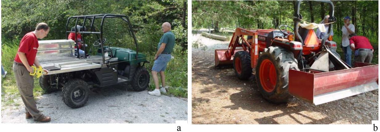
Figure 2. a. Four wheel ATV emergency vehicle (1670 lb.) b. Small construction tractor with box blade and front end loader (5700 lb).
