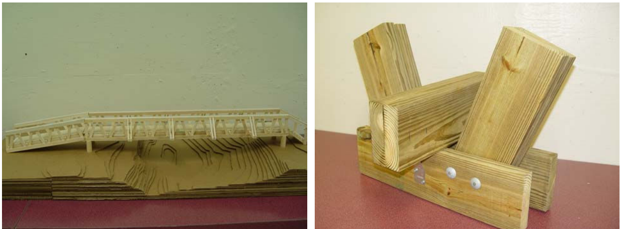
Figure 3. Student created physical models illustrating alternatives for the approaches and connection details of the superstructure of the proposed bridge.
