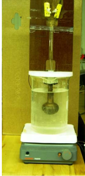
Figure 2: Experimental set-up. A hot sphere (near 420 C) dipped in near boiling water.
