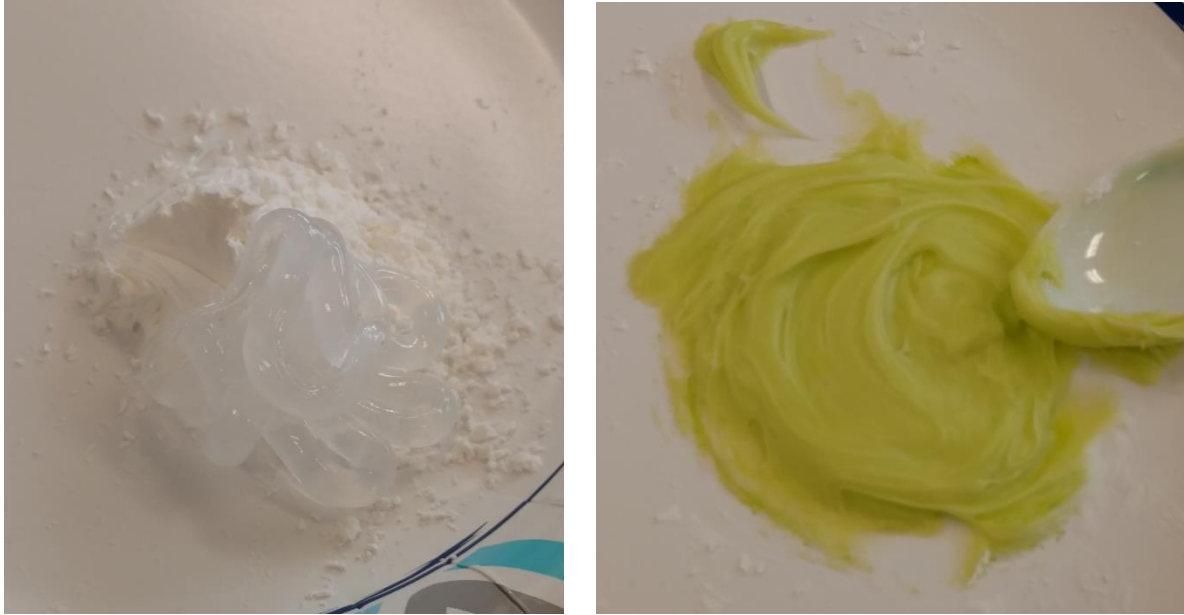
Figure 8: Silicone and cornstarch before and after mixing. Yellow food was added for aesthetics.
