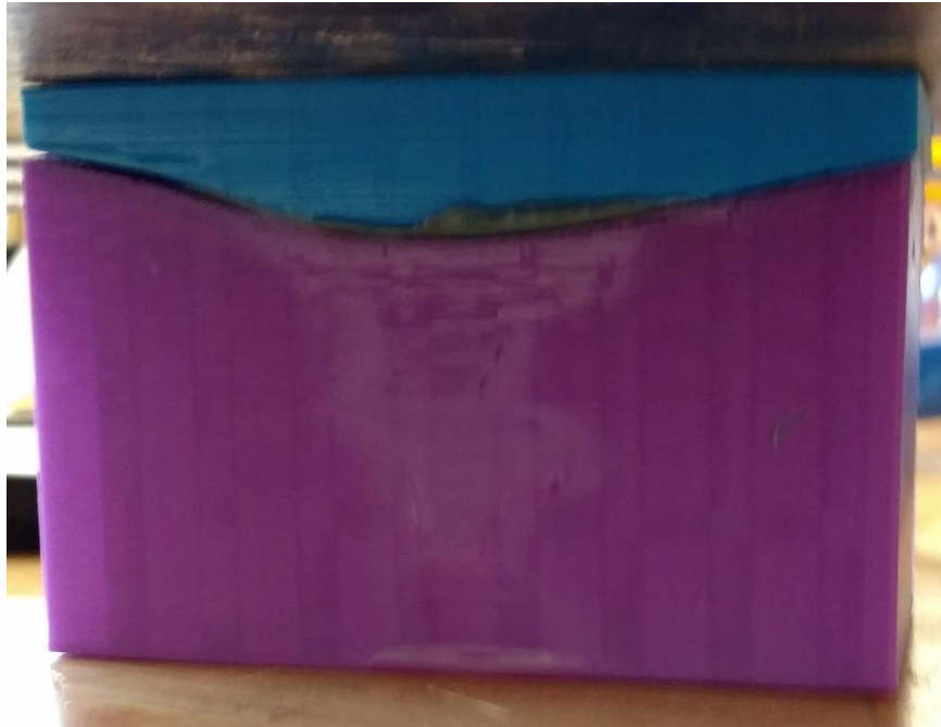
Figure 10: Completed mold with weight on top, allow at least 12 hours to cure.
