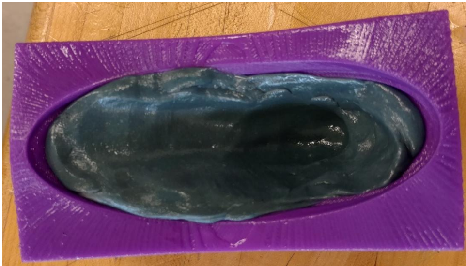
Figure 9: Insertion of silicone into mold, ensure the material is spread evenly with no holes.
