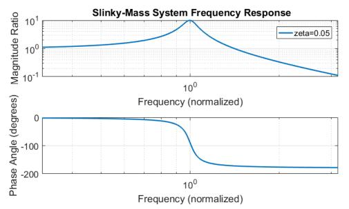
Figure 20: Frequency Response Plot for an Underdamped second order system
