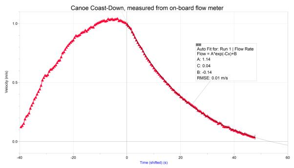
*Figure 4: Canoe Coast-down starts at time 0. Data collected from onboard flowmeter. Exponential curve fit displayed as black line.*
