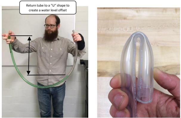
Figure 11: Creating the initial condition Figure 12: To restrict airflow fold over the tube
