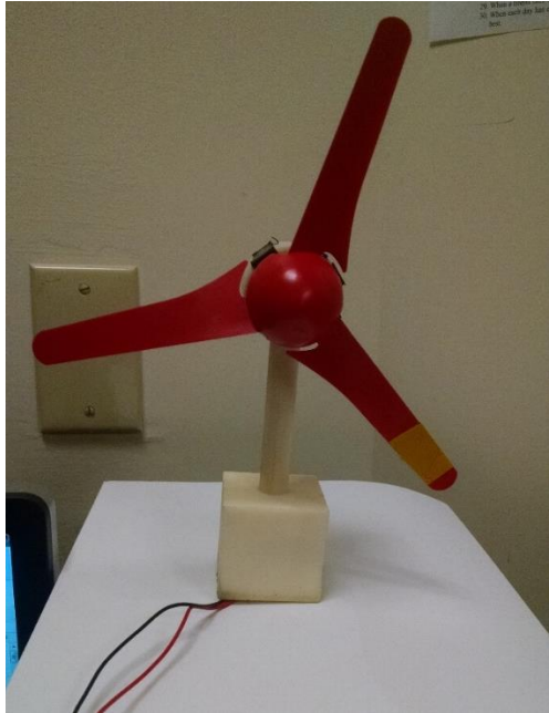
Figure 2: Horizontal axis wind turbine with custom 3D printed base
