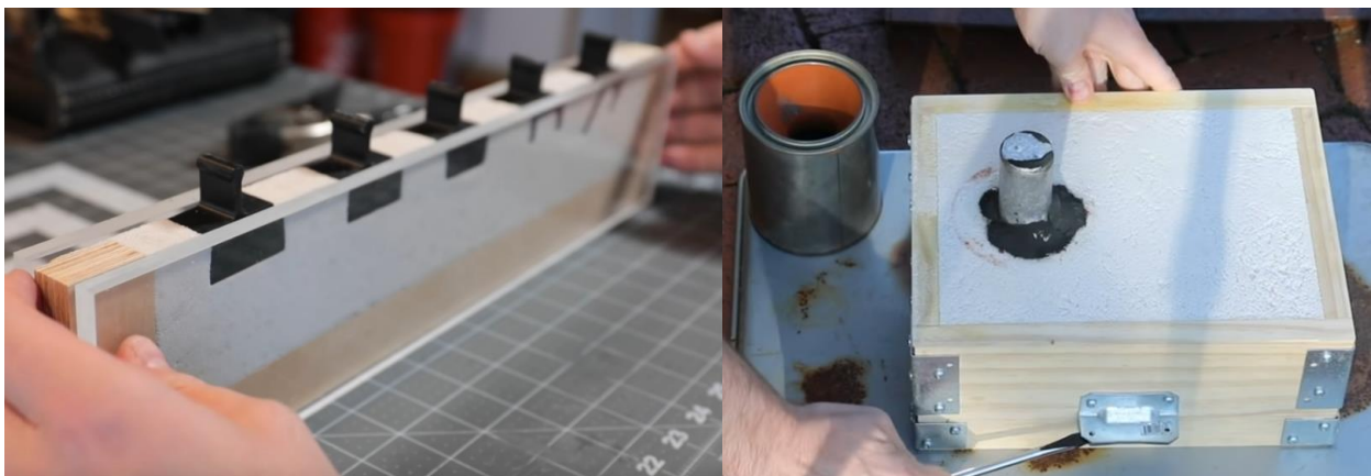
Figure 3. Physical teaching aid demonstrating the concept of a draft angle (left) and no-bake casting method after an aluminum casting is completed (right) [10].
