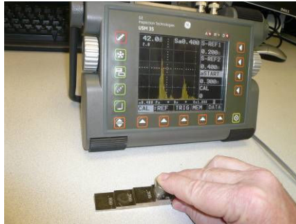
Figure 2. Calibration of the flaw detectors using a straight-beam probe.
