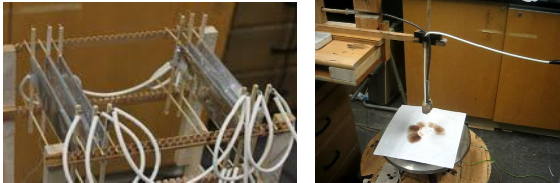
Fig. 2 Experimental apparatus designed and built by students for investigation of corona wind (a) Experimental setup for observing a new electro-spray regime of ferrofluids (a)
