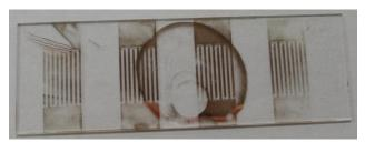
Figure 6: Circuit pattern etched from copper coated slide.
