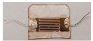
Figure 7: Photoresist coated devises with electrodes (2 will be needed to create one device).
