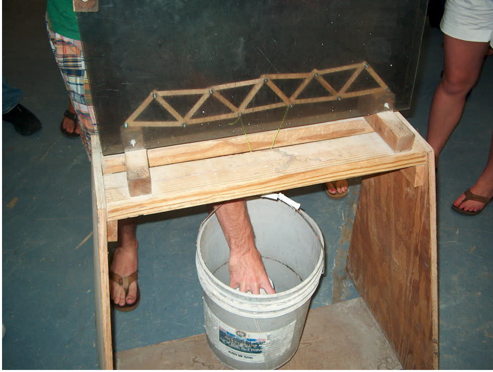
Figure 3. Loading of truss bridge
