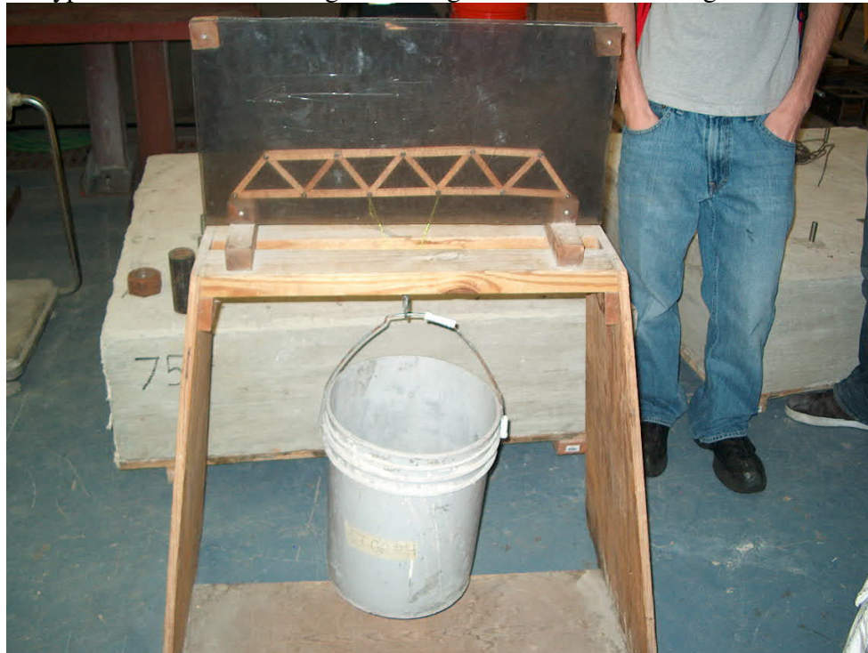
Figure 2. Typical student truss bridge with small craft sticks in testing frame
